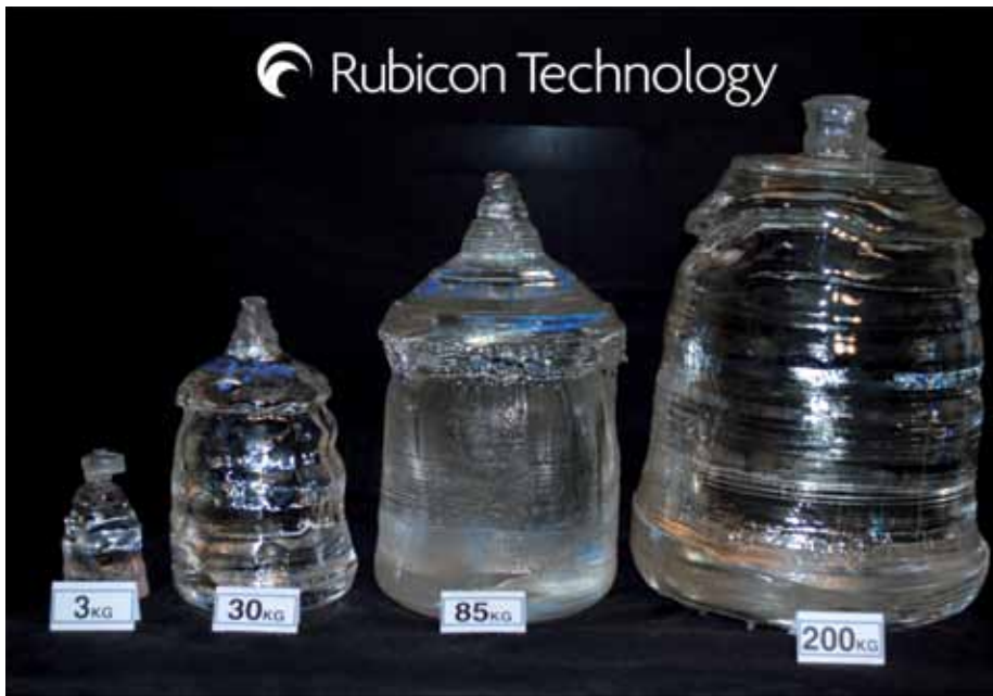
Sizing up: Rubicon's ES2 sapphire crystal growth technology has progressed from making 3kg boules suitable for 2-inch wafers to 200kg boules from which wafers larger than 12-inch diameter can be made (Courtesy of Rubicon)
