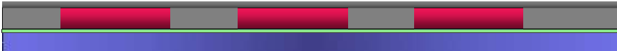
7) de-bonding and foil removal, wafer is turned upside down, plasma cleaning and planarization of the front side
