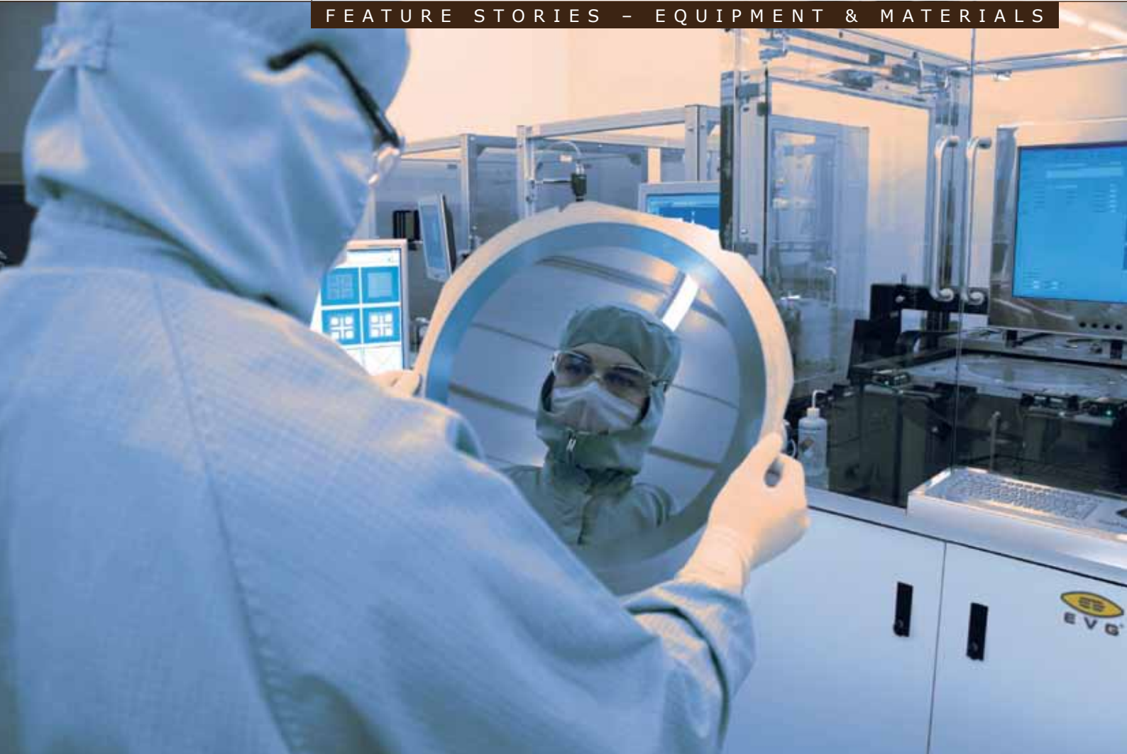
Thin Si Wafer on Carrier (Courtesy of EVGroup)
