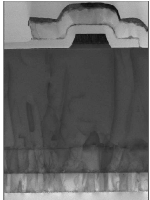
TEM view of the GaN layer (Courtesy of System Plus Consulting)
